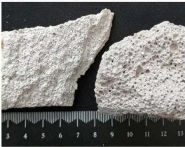
Photo of RAAC samples showing variability of the material
